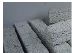
Plastic Waste into Hollow Concrete
